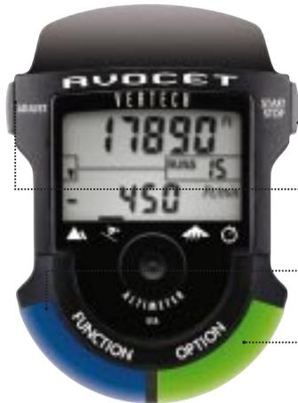
Accessing different functions is simple. The four icons directly below the LCD correspond to the four primary functions. Pressing the purple function button on the left side of the Vertech presents the primary functions, and an identifying bar appears on the LCD above the icon of the chosen function. To present options of a displayed function, press the red option button on the right side.
