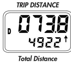
**TRIP DISTANCE (D)**. Displays Trip Distances up to 1999.9 miles or km in .1 increments in the upper numbers. Reset by pressing both buttons.
