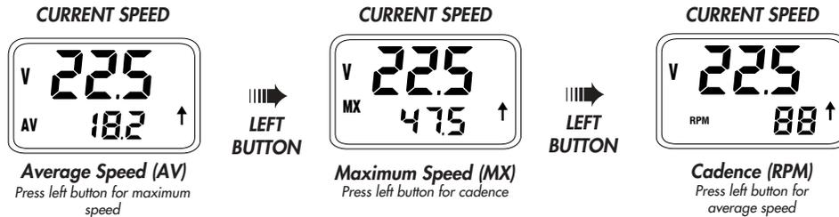
**CURRENT SPEED (V)** displays current speed up to 128 mph or 206 km/h.
