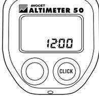
*Press the right button to move from one setup function to the next.*
