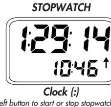
**STOPWATCH**. Upper numbers show elapsed time. Press the left button to start or stop. Shows times up to 1 hour, 59 min, 59 sec, then resets and resumes counting. Reset by pressing both buttons.
