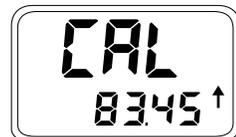
*Left button increments calibration numbers up or down depending on arrow direction*
