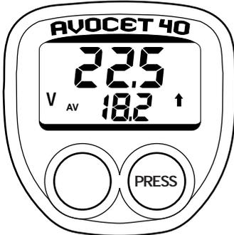
CURRENT SPEED is shown in the upper display. Press the option (left) button to select Average Speed (AV), Maximum Speed (MX) or Cadence (RPM).
