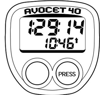
STOPWATCH is in the upper display and Clock in the lower display. Press option (left) button to start and stop the stopwatch.
