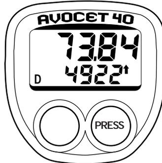
TRIP DISTANCE is shown in the upper display and Total Distance in the lower display.
